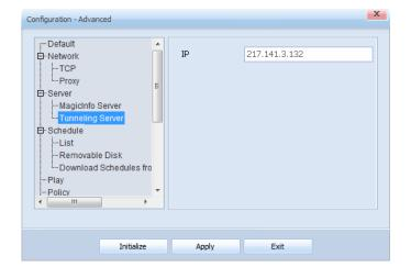
Enter in the IP or URL address of the tunneling server that will be used on the VNC.
